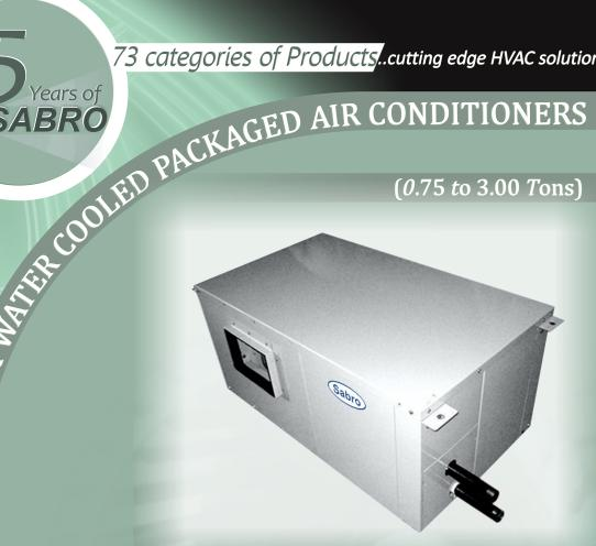
The Mini Water Cooled Packaged Air Conditioners are designed for installation within the conditioned room. The heat of conditioned room is removed through condenser water by means of a cooling tower. The use of cooling tower is essential with these units.
