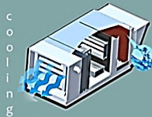
DX-Evaporating cooling with Diesel Furnace
